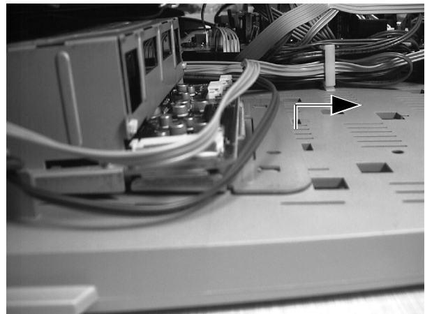
Figure 4-2 DVD lock plate removal.
