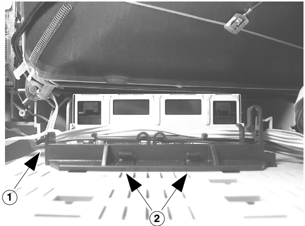
Figure 4-2 DVD lock plate removal.
